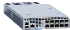
T-XR45 10-S / CISCO SWITCH (ESS) 9300 1U Switch Sled Supports (10) 10Gb SFP+ Ports
