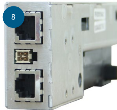
Connect two data cables and one sensor emitter cable
