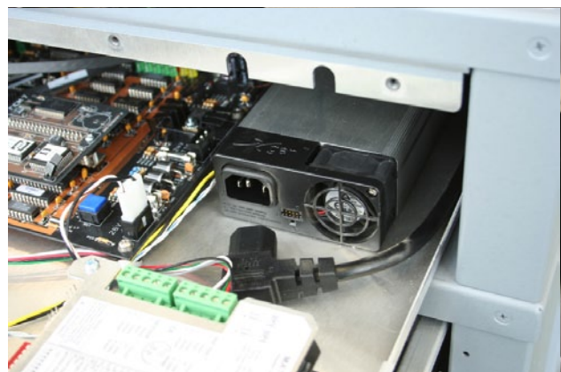
Remove two data cables from right side of Interface Board
