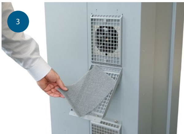
3 Remove filter material and replace with a clean piece
