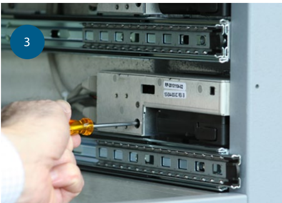
Loosen drawer module retaining screw (#1 Phillips bit)
