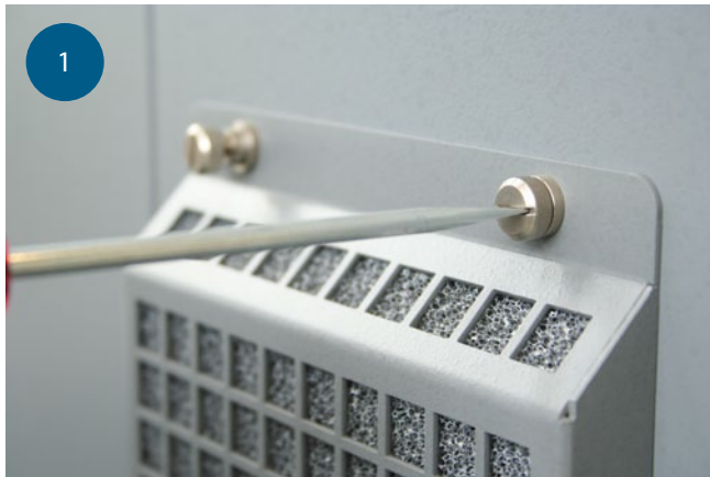
1 Loosen thumbscrews (might require screw driver to start)
