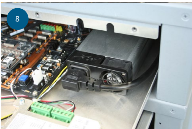
Remove one LAN cable from right side of top board
