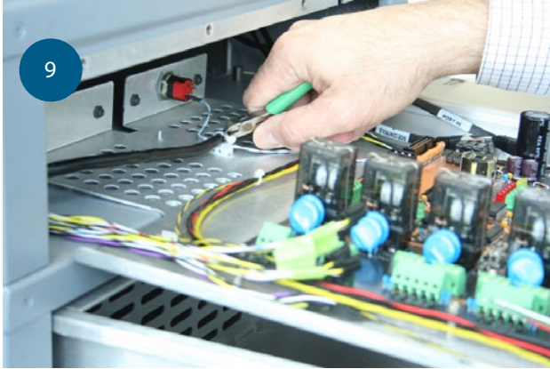
9 Cut wire ties on AC line cord
