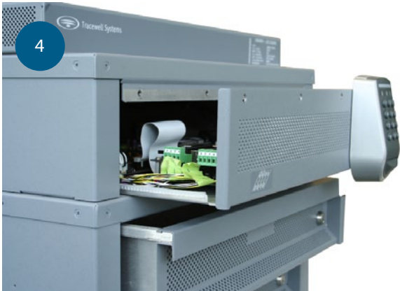
Pull Electronics Bay out about 4"
